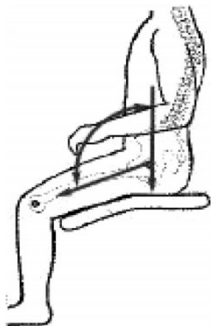
Figure 6: The 2-part curved seat pan design prompts forward leaning and increases the thigh torso angle. This design preserves lumbar lordosis, or the curving of the lower back.
